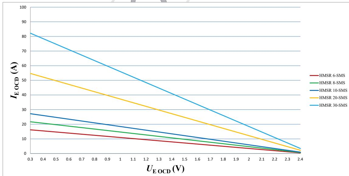
$$I_{E\text{ OCD}} = \frac{(V_{ref} - U_{E\text{ OCD}})}{G_{Th}} \times 1000 \quad U_{E\text{ OCD}} = \frac{R_E}{R_E + R_{ref}} \times V_{ref}$$
